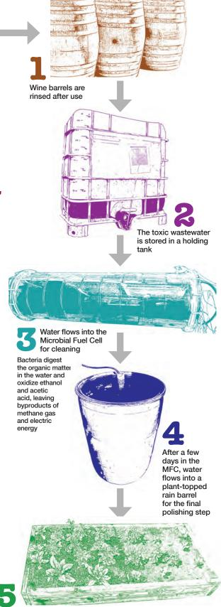
When finished, the water is used to irrigate an on-site garden
